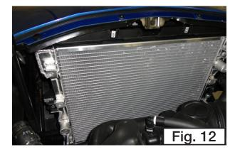
14. Move the radiator into the stock mounting location. Using the two 13mm bolts attach the radiator to the car (Fig. 13).
